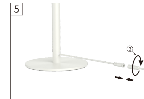
Plug the male end of the power output cable into the light pole input cable, rotate it 90° and fasten it.
