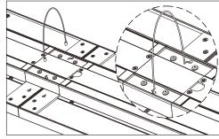
Install the wire rope onto the connecting block, making sure that the wire rope does not slip out of the mounting hole
