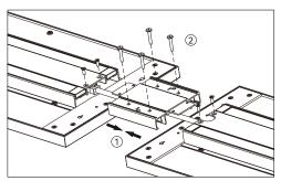
Secure the cascade block to the lamp body with screws.
