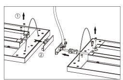
Loosen screw 1 as shown in the figure and remove the end cover on the side to be connected
