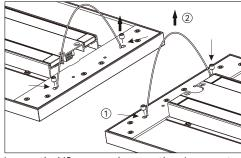
Loosen the M5 screw and remove the wire rope at the splicing end.
