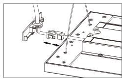
Remove the power cord at the desired link by disconnecting the pairs of terminals.
