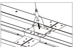
Lock the screws, adjust the wire rope to the appropriate height, tighten the screws, and secure the wire rope.
