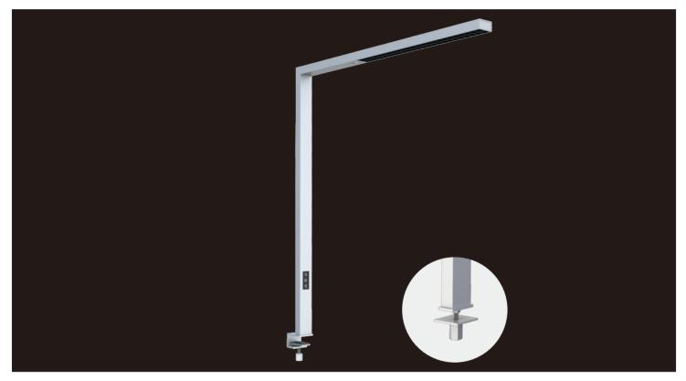
With extremely simple design and excellent craftwork, exquisite appearance looks with rich of texture. Lamp is designed with special Direct/Indirect lighting and 50°(Direct) & 110°(Indirect) beam anale. Collocated with micro reflector and anti-alare cover, UGR value is as low as 6. Adopting DIY assembly structure, there is no need of professionals. With special bracket, light can be easily fixed at desk edge and is convenient for using.
