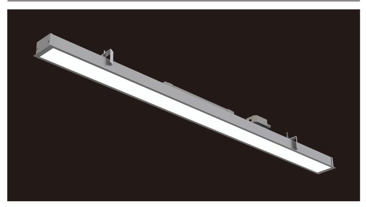
Simply and reasonable structure design with excellent craft work. Appearance with rich texture. flexible prism mask design, no light leakage from seams, Reliable heat dissipation system. 5 years warranty. Typical value up to 110lm/W with flicker freely. 1-10V and Dali synchronous dimming, support CASAMBI wireless system. Profile aluminum, Recessed installation, Easy & Fast.
