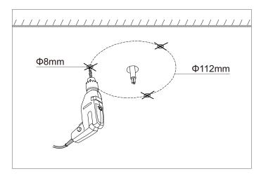
1.Punch three holes (size:Φ8mm\*50mm) at the position of three equal parts on a circle (diameter :112mm) in the ceiling.
