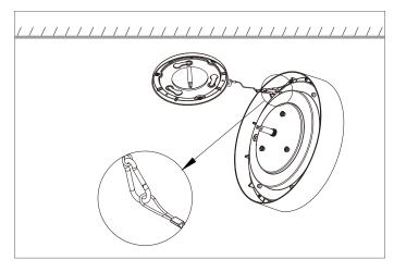
4.Put the safety rope around the metal clip of the lamp body, then connect the cables (ensure the power is off and input AC 200-240V).
