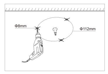
1.Punch three holes (size:Ф8mm\*50mm) at the position of three equal parts on a circle (diameter :112mm) in the ceiling.
