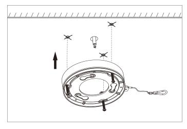
3. Fix the base to the ceiling with self-tapping screws.
